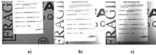
Fig. 19. Label image: a) without illumination; b) with direct lighting; c) with indirect lighting.
