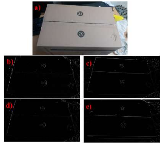
Fig. 12. Results of the Sobel operator: a) Box image without processing; b) Result of vertical Sobel operator; c) Result of horizontal Sobel operator; d) Result of vertical Prewitt operator; e) Result of horizontal Prewitt operator.
