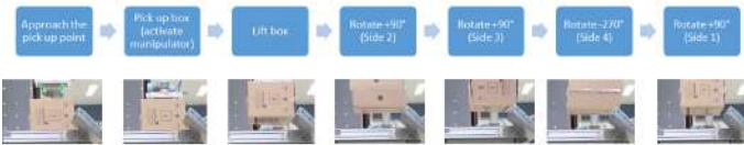
Fig. 9. Sequence for quality control manipulation with Cobot.
