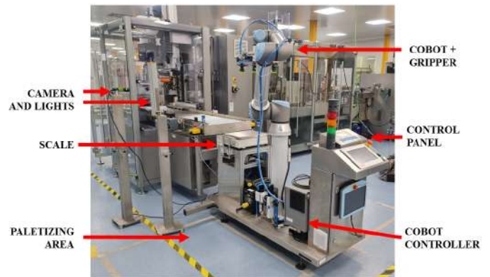
Fig. 7. Automatic mechatronic palletizing system implemented.
