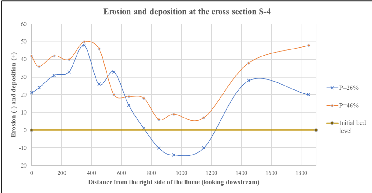
Figure 16. Final bed levels in cross section S-4. Notice that bed levels in the 46% permeability test was greater than in the 26% permeability test. Dimensions are shown in millimeters.
