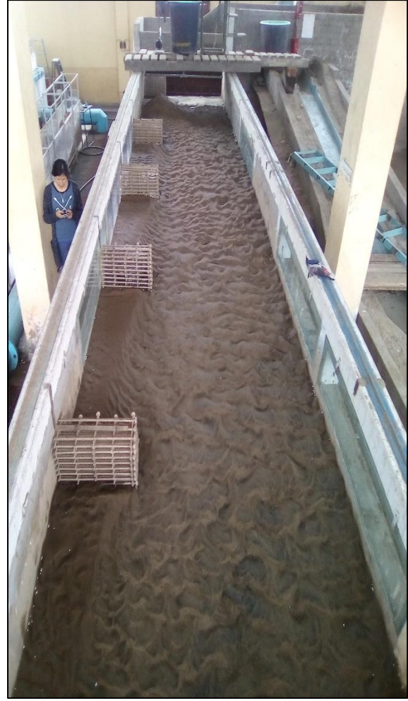
Figure 13. Scour and deposition patterns and bedforms after the 46 % permeability test was concluded.
