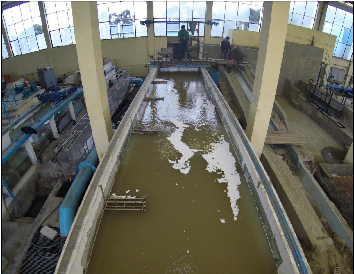
Figure 6. Test conditions during the 46 % permeability tests. Polystyrene balls were added for visualizing the flow field.
