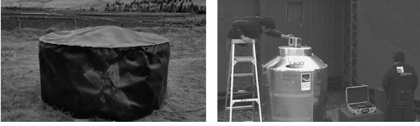
Fig. 1. The two peruvian WCDs of the LAGO project, one in Huancayo (left): 2,4 m diameter - 0,9 m height, and the other in Peru's Antarctica Camp (right): 1,2 m diameter - 1 m height, used in this work.
