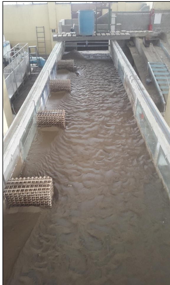
Figure 12. Scour and deposition patterns and bedforms after the 26% permeability test was concluded.
